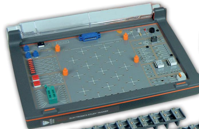
Discrete electronic components mounted on carriers
