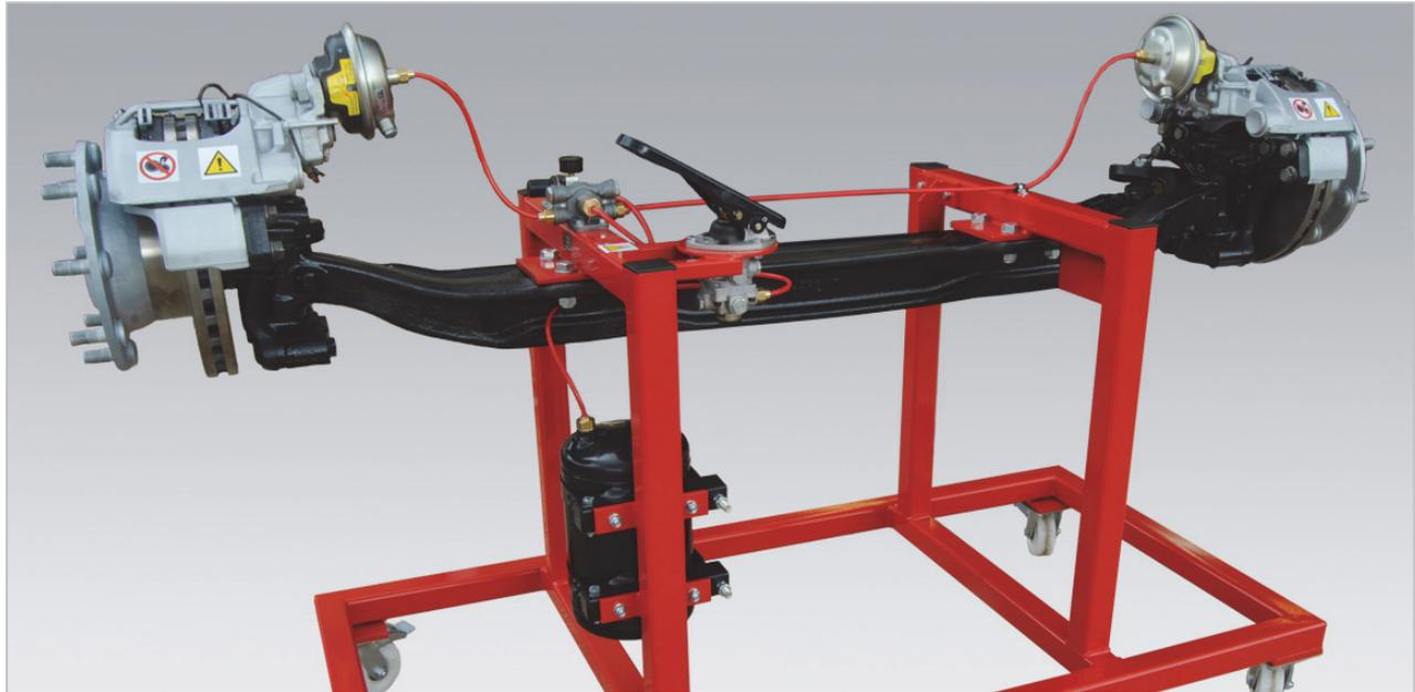
Fully operational heavy vehicle front axle - complete with disc air braking system, using single line air pressure to operate the disc brakes via the foot brake and treadle valve.
