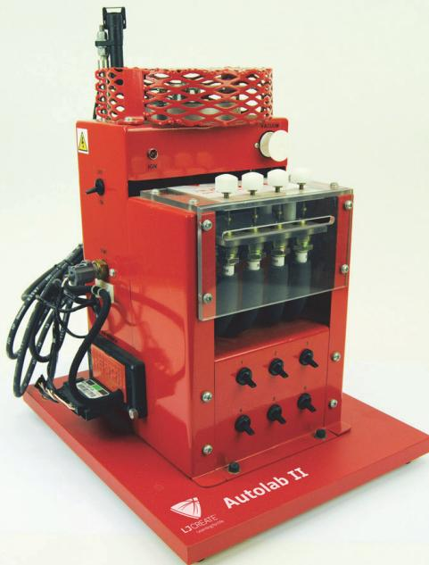
This real component trainer provides the instructor with a working distributorless ignition system for group or whole-class demonstration.
