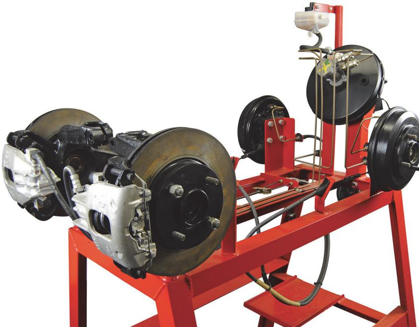
This real component-based trainer provides students and instructors with the opportunity to demonstrate and investigate the operation of a typical automotive braking system. The trainer is designed to allow access to disc and drum brake components, as well as providing the opportunity to understand the operation of the hydraulic circuit.
