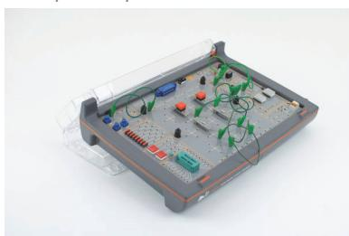
When in use, the cover folds back to provide an angled support for the unit. With the cover closed, trainers become stackable for easy storage.
