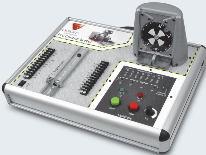
The 291-01 training system offers a platform that enables students to perform a comprehensive range of programming tasks culminating in the control of the unit using an industrial programmable logic controller (PLC).
